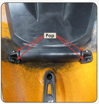
5. Insert the Cherry Rivets(B) into each hole and pop with your Rivet Gun.
